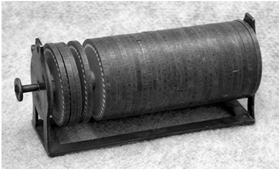
Figure 5-2: The Jefferson Disk, one of the earliest cryptographic machines
