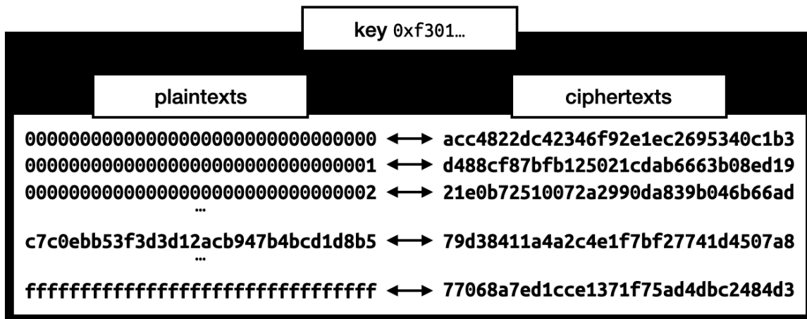
Figure 4.2 A cipher with a key can be seen as a permutation: it maps all the possible plaintexts to all the possible ciphertexts.
