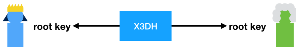
Figure 10.16 Naively, a post-X3DH protocol could simply use the output of X3DH as a session key to encrypt messages between Alice and Bob.
