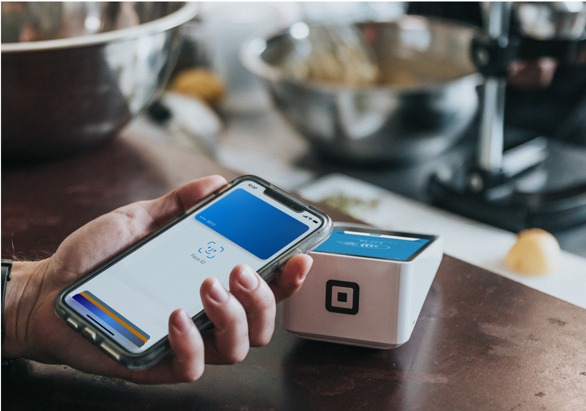
Figure 11.17 Near Field Communication (NFC) is a set of wireless protocols that allow devices to communicate when brought within 10cm of each other. The protocol is most commonly used by "contactless" payment systems (mobile payment applications like in the picture, contactless credit cards, and so on).
