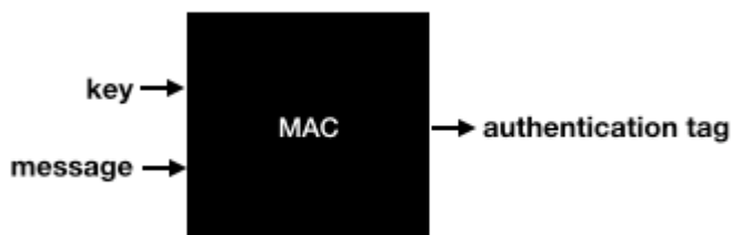
Figure 3.3 The interface of a message authentication code (MAC). The algorithm takes a secret key and a message, and deterministically produces a unique authentication tag. Without the key, it should be impossible to reproduce that authentication tag.
