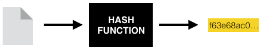
Figure 2.2 A hash function takes an arbitrary-length input (a file, a message, a video, and so on) and produces a fixed-length output (for example, 256 bits for SHA-256). Hashing the same input will produce the same digest or hash.
