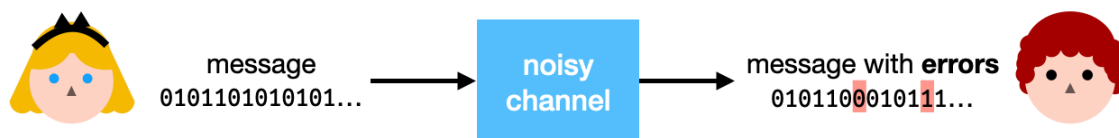
Figure 14.12 Physical noise can happen naturally for all sorts of reasons. This physical phenomenon can impact the integrity of data being transmitted or stored.
