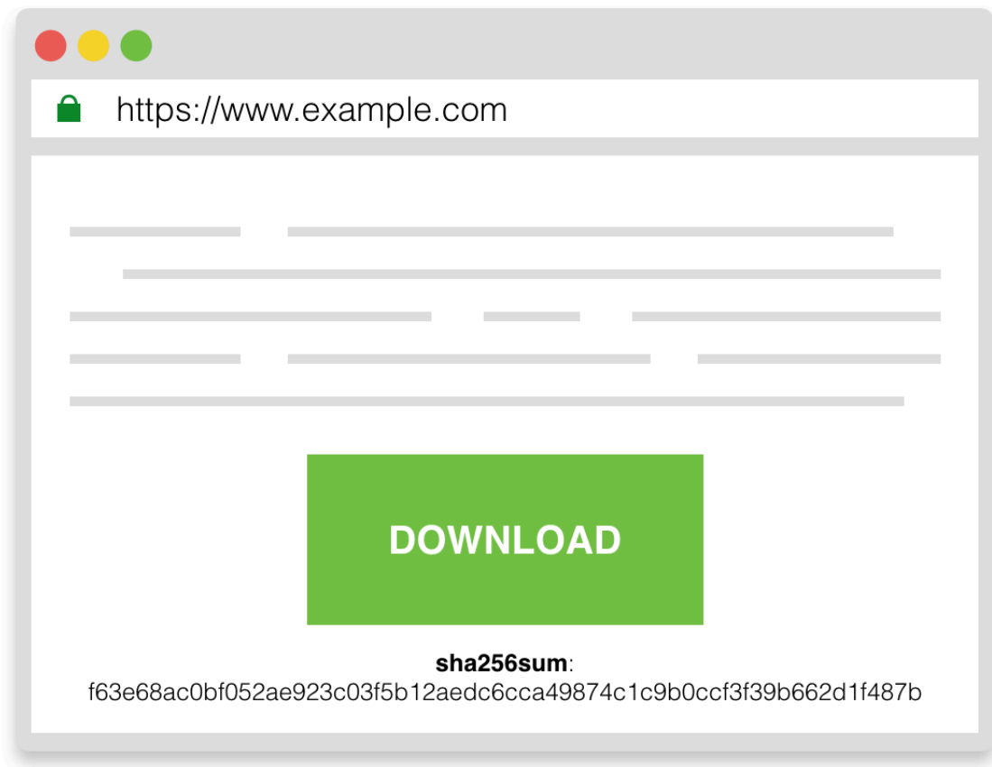
Figure 2.1 A webpage linking to an external website containing a file. The external website cannot modify the content of the file, because the first page provides a hash or digest of the file, which ensures the integrity over the downloaded file.
