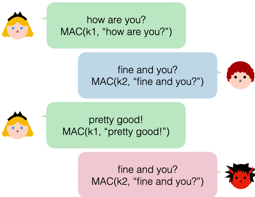
Figure 3.5 Two users sharing two keys k_1 and k_2 exchange messages, along with authentication tags. These tags are computed out of k_1 or k_2 depending on the direction of the messages. A malicious observer replays one of the messages to the user.
