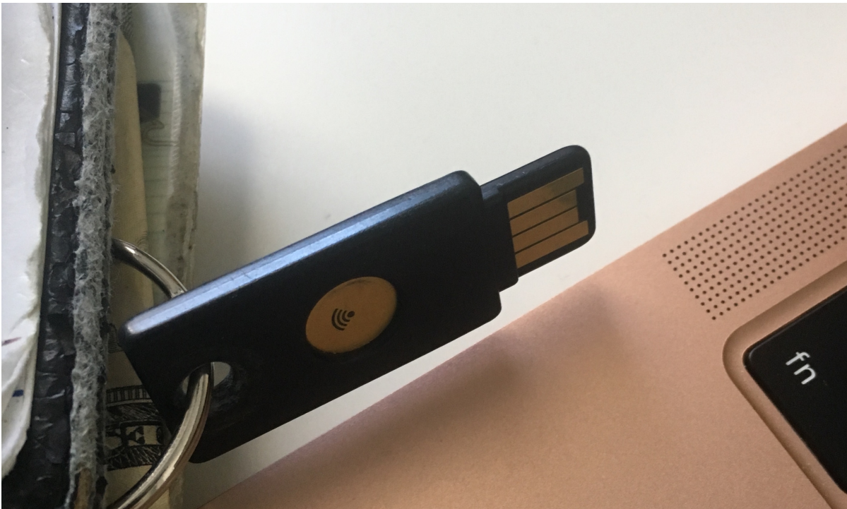
Figure 11.14 A YubiKey is a security key, one type of "roaming" authenticator that can be used with FIDO2. Its role is to store private keys associated with different applications. It is inserted in the USB port of a computer (roaming authenticators can communicate with a platform via USB, Near Field Communication (NFC), or Bluetooth) and will not perform any cryptographic operations unless triggered by the touch of a finger on its gold metal button.
