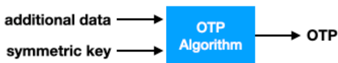
Figure 11.10 A one-time password (OTP) algorithm allows you to create as many one-time passwords as you want from a symmetric key and some additional data. The additional data is different depending on the OTP algorithm.
