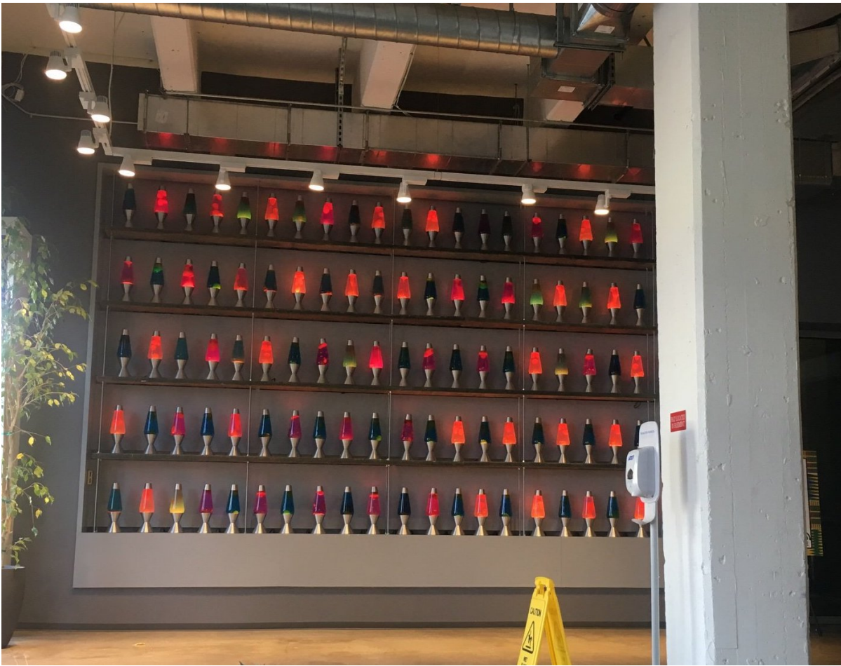
Figure 8.1 A picture I snapped during one of my visits to the headquarters of Cloudflare in San Francisco. LavaRand is a wall of lava lamp, which are lamps that produce hard-to-predict shapes of wax. A camera is set in front of the wall to extract and convert these images to random bytes.
