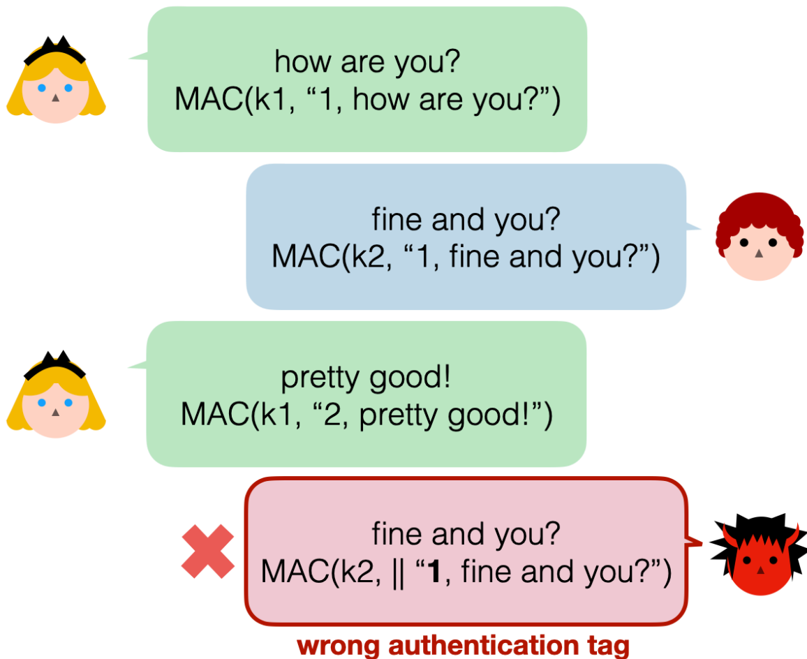
Figure 3.6 Two users sharing two keys k_1 and k_2 exchange messages, along with authentication tags. These tags are computed out of k_1 or k_2 depending on the direction of the messages. A malicious observer replays one of the messages to the user. Since the victim has incremented his counter, the tag will be computed over 2, fine and you? and will not match the tag sent by the attacker. This will allow the victim to successfully reject that replayed message.
