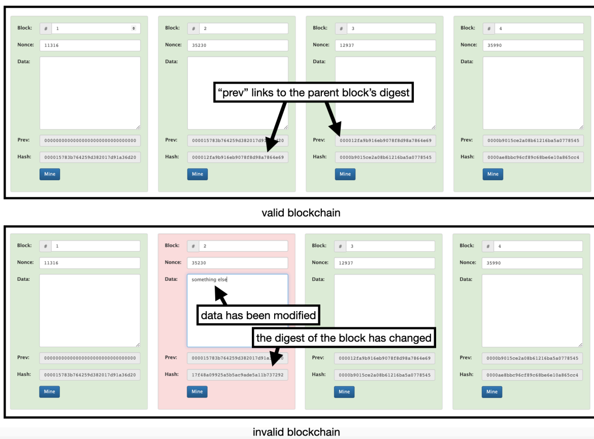
Figure 12.4 On https://andersbrownworth.com/blockchain/blockchain one can interactively play with a toy blockchain. Each block includes its parent's digest, and each block contains a nonce found randomly that allows its digest to start with 4 zeros. Notice that this is true for the top blockchain, but the bottom one contains a block (number 2) that has been modified (its data was initially empty). As the modification changed the digest of the block, it is no longer being authenticated by subsequent blocks.
