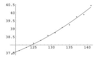
**Fig. 8.** Bits required to locate the private key for  $q = 1024, d_f = 29$  (tail).
