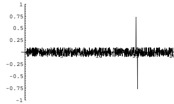
Fig. 1. Simulated correlation function g(t) between the points 4P_i and power consumption C_i(t) when d_{\ell-2} = 0 . A peak is observed corresponding to the computation of 4P_i inside the card.
