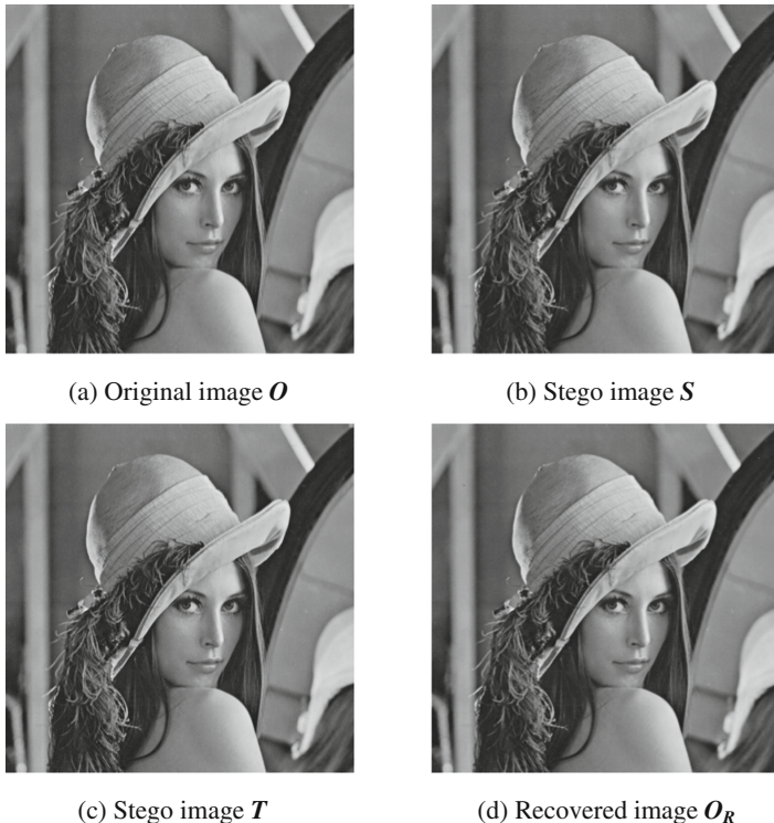
Fig. 2. Experiments for the Lena with a size of 512 \times 512 (256-gray): (a) the original Lena image O , (b) the stego image S using the proposed PM method (1.50 bpp), (c) the stego image T based on directed LSB embedding (0.67 bpp), (d) the recovered image O_R without any loss.
