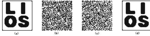
Fig. 1. A 2 out of 2 VCS_{XOR} where (a) is the original image, (b) and (c) are the shares, (d) is the recovered image from (b) and (c).
