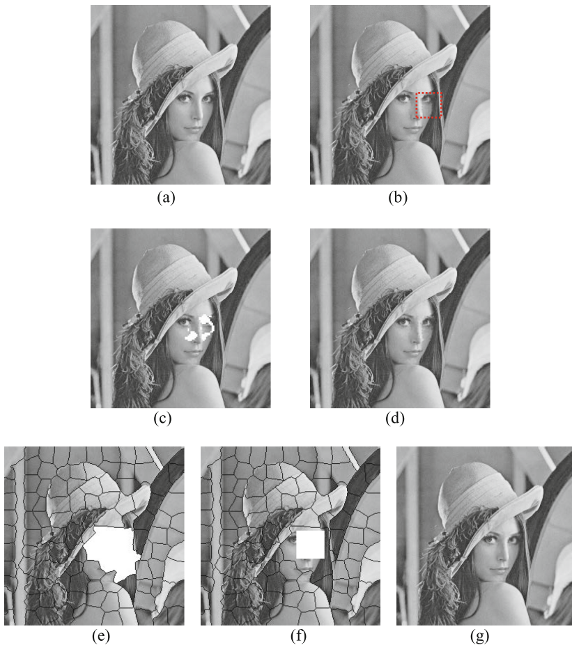
Fig. 7. Original image and tampered detection for “Lena”. (a) Watermarked image, (b) The tampered image under VQ attack, (c) Tamper detection results and (d) Recovered image by He’s method [9], (e) The authentication based on superpixels, (f) Precise detection and (g) the recovered image by the proposed method
