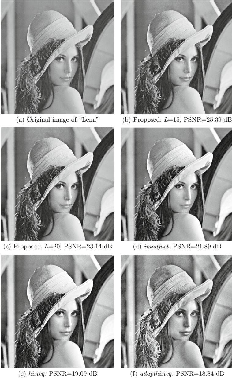
Fig. 5. Experimental results with the proposed algorithm and three matlab functions: (a) Original image of "Lena"; (b) Proposed algorithm with L=15 : PSNR=25.39 dB; (c) Proposed algorithm with L=20 : PSNR=23.14 dB; (d) imadjust with the default setting: PSNR=21.89 dB; (e) histeq with the default setting: PSNR=19.09 dB; (f) adapthisteq with the default setting: PSNR=18.84 dB.
