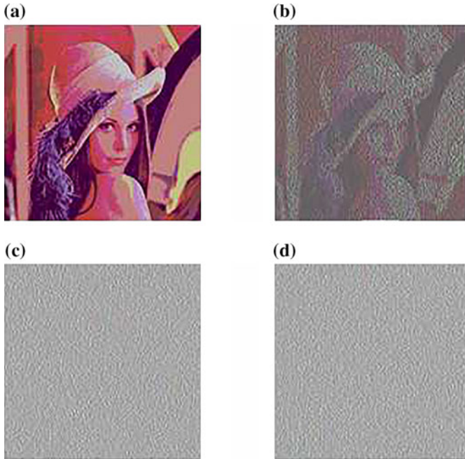
Fig. 5.1 Experimental results of the color (2, 2)-VCS with no pixel expansion in the visual cryptography model of Naor and Shamir (size of the secret image is 256 \times 256 ). a Original secret image; b Resulting image by superimposing (c) and (d); c Encrypted shares; d Encrypted shares
