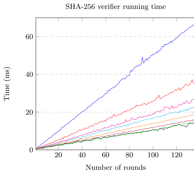
Fig. 10. Relation between the running time ( without disk writing operations ) and the number of rounds for the SHA-256 verifier, average over 100 runs.
